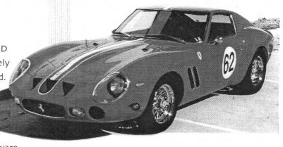
and the doors. However, Ed took the time to remedy this problem by filling the gap with fiberglass and resin then cutting his own "gap" in. The final product is a perfect body panel fit. Nevertheless, this attention to detail did not stop with body work and paint. To name a few, the interior was retrofitted, the suspension upgraded, the exhaust system addressed, and a completely blueprinted and rebuilt engine and transmission.
